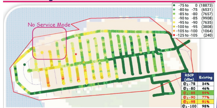
Existing Sites Pre-Drive Test RSCP Result
